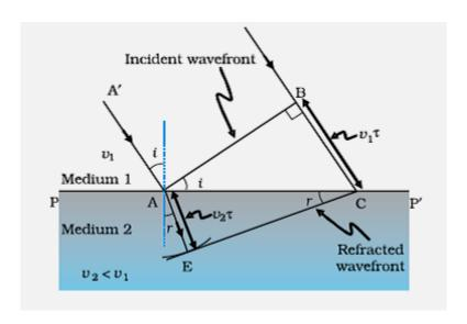
Let t be the time taken by the wavefront to travel the distance BC in rarer medium and AE in the denser medium
